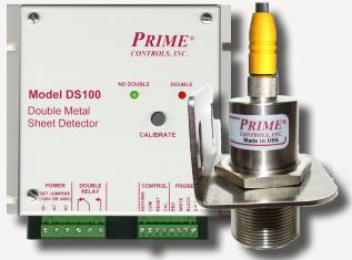
The DS100 Double Sheet Detector is simple to calibrate. Simply place a metal sheet on the front of the probe and push the calibrate button once. With one push of the button, the DS100 automatically measures the thickness, calculates its double value and sets the reject threshold midway between the single and double values. It's that easy.
